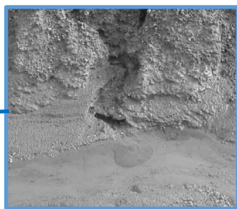
湧水箇所① 粘性土と砂質土の互層
